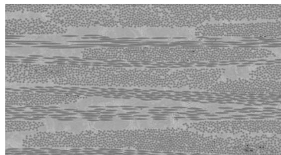
Microstructure of oxide composite ceramic with Al<sub>2</sub>O<sub>3</sub> fiber reinforcement @ CME
