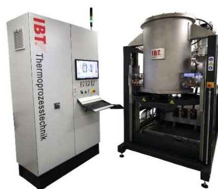
Vacuum furnace of the ThermoLine-VAC series @ IBT
