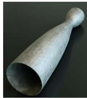
Laval nozzle of C/SiC (LSI) @ HTL
