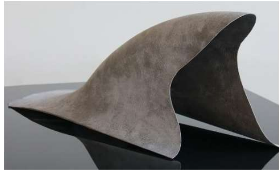
Partial segment of a mixer made of GMC (geopolymer matrix composite) with basalt fibers @ HTL
