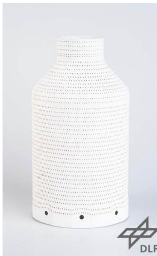
Combustion chamber made of alumina CMC by winding technology @ DLR-WF
