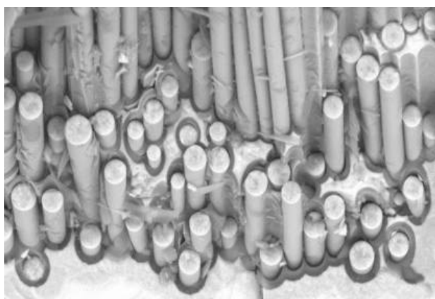
Fracture surface of a tough CMC @ DLR-BT
