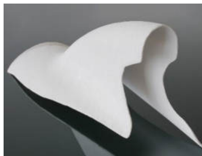
Partial segment of an OFC mixer made from silica fibers and oxide ceramic matrix @ HTL
