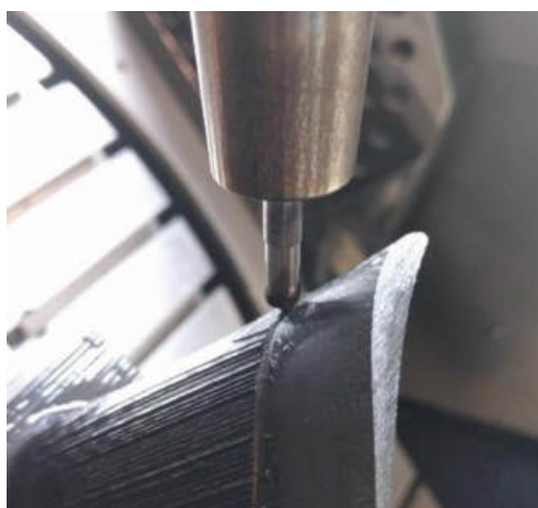
5-axis machining turbine blade @ Gühring
