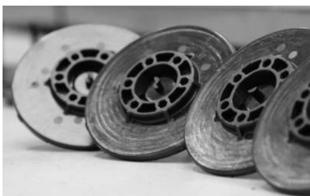
C/C-SiC brake discs for GoCarts via injection moulding and LSI @ TUC-TKV
