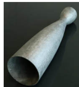
Laval nozzle of C/SiC (LSI) @ HTL
