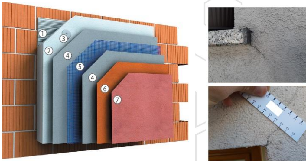
Figure: left - 1 Primer, 2 Thermal insulation, 3 Anchor, 4 Base coat, 5 Reinforcement mesh, 6 Primer, 7 Top coat; right - crack examples
