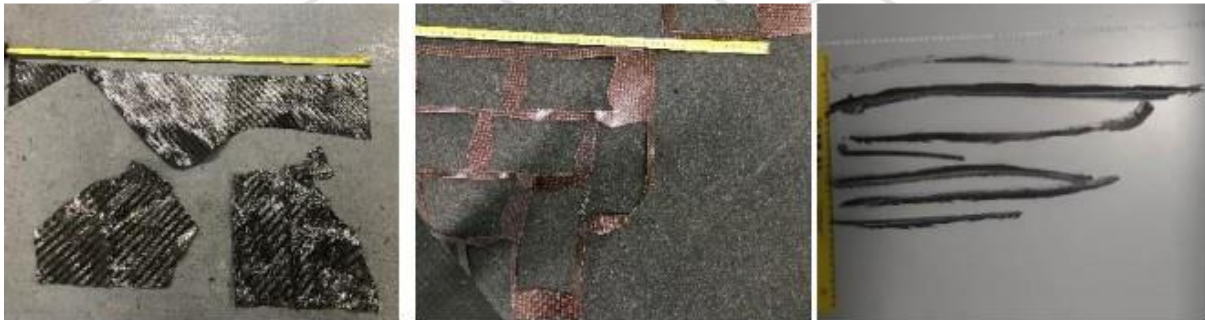
Figure 1: hybrid CF/GF reinforced epoxy scraps from manufacturing process.
