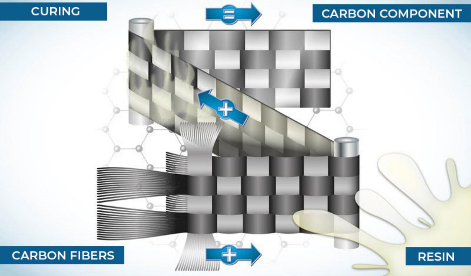
Carbon is a fiber composite material. A fiber composite material is produced by combining two components to create a completely new material. This has better properties than the individual components themselves due to the interaction of the two components. Generally, reinforcing fibers are embedded in a plastic matrix (e.g. epoxy or polyester resin) during production. For example, carbon (CFRP is produced) or glass (GFRP is produced) are used as the fiber material for this purpose.
